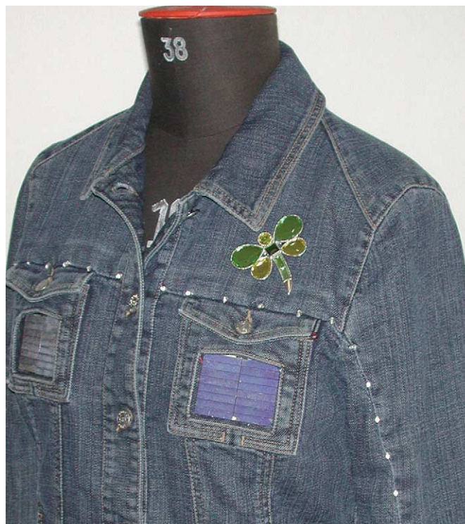
Fig. 6 BOGNER/MUSTANG denim jacket including a small-area photovoltaic add-on designed for the Avantex fair in 2005. Brittle c-Si cells are fixed onto a rigid metallic backplane that ensures mechanical stability, with their front and back contacts series-connected at the same time like roofing shingles. Two modules, each of 16 cells, power blinking or walking lights along the arms of the jacket where high-brightness white light emitting diodes are incorporated. (Courtesy of MUSTANG 49 .)
