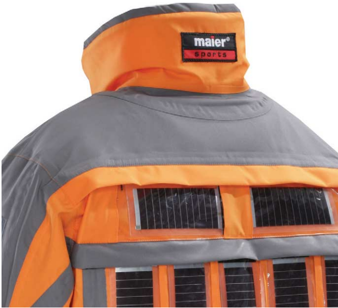
Fig. 1 Prototype of a winter outdoor jacket with ipv. This jacket was developed by Maier Sports 6 , with support from the Institut für Physikalische Elektronik and other partners in the German SOLARTEX project 7 . The jacket was first presented in Munich at the International Trade Fair For Sports Equipment and Fashion (ISPO) in January 2006. It comprises nine amorphous Si solar modules from Akzo Nobel 8 with a maximum power output of 2.5 W under full sun. (Courtesy of Maier Sports.)
