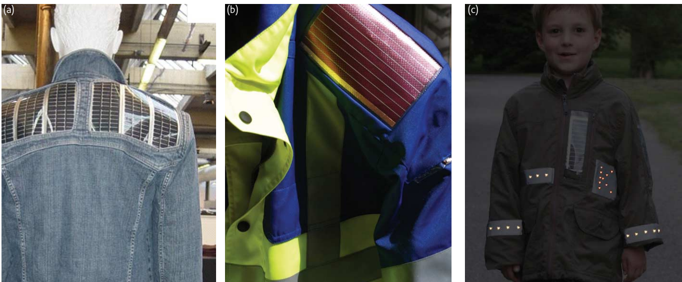
Fig. 12 Examples of SOLARTEX 7 prototypes for different applications. (a) The BOGNER/MUSTANG 49 jacket provides a universal socket and energy buffer for operating and charging USB-compliant devices. Iowa Thin Films modules 44 deliver a maximum power of 2.5 W. Three hours of full sun enable 40 hours of mp3 operation. (b) In the TEMPEX jacket 62 , bright photovoltaic-powered warning lights supplement the built-in passive safety features, e.g. for street construction workers. (c) Using photovoltaic power harvested during the day, light-emitting diodes enhance the visibility of children at night in this KANZ coat 63 . (Courtesy of Institut für Textil- und Verfahrenstechnik 65 ).
